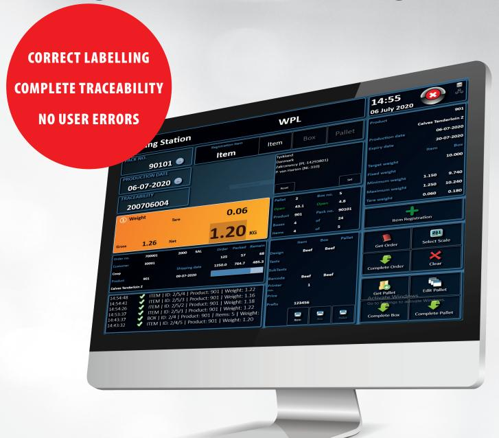
ScanPlant WPL is an intelligent software system that ensures that the products are labelled with the correct data. The system registers all of the traceability data through all production processes and has an automatic summation of data function, which gathers data for the next packaging level – from item to box and from box to pallet.
