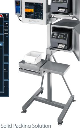
ScanPlant WPL can also be used at Scanvaegt's packing stations for weighing, packing and labelling with individual weight and weight/price barcodes. The packing station, which consists of Scanvaegt's solid industrial weights, pt9000 industrial terminal and printer, can also be supplied as a waterproof solution with a stainless-steel cabinet for a printer
